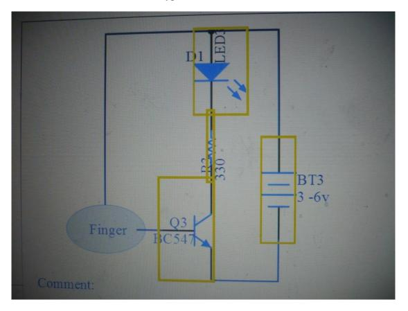
Fig. 2 the design of the circuit, presents battery with voltage 3 to 6 volts, LED, resistance 330 kilo Ohm, transistor type BC 547 and finger
