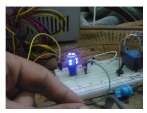
Fig.3. illumination of the LED due to contact with alive finger touches it
